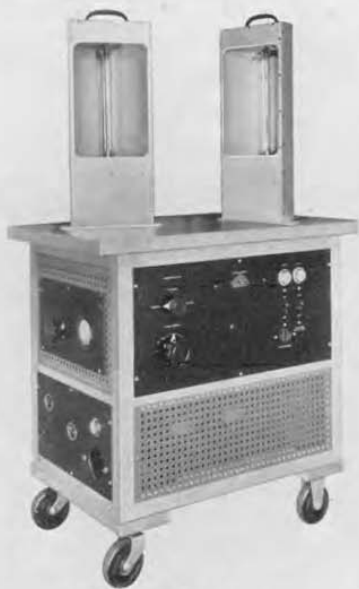
FIGURE 2. Control unit of the TYPE 621-H Edgerton Power Stroboscope showing the mercury lamps. The complete stroboscope consists of this unit and a 10-kw motor generator
