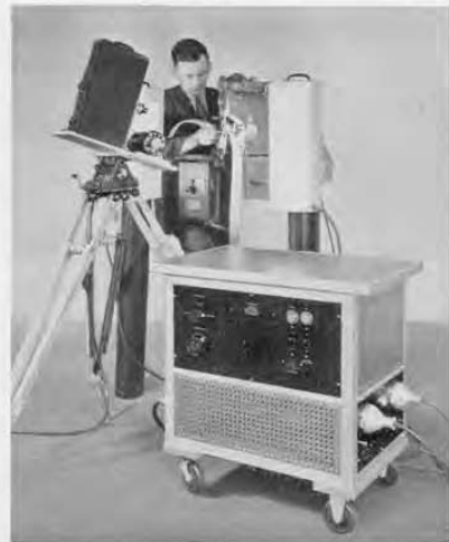
FIGURE 1. TYPE 621-H Stroboscope and TYPE 651-A Camera set up to photograph a machine for stitching leather
